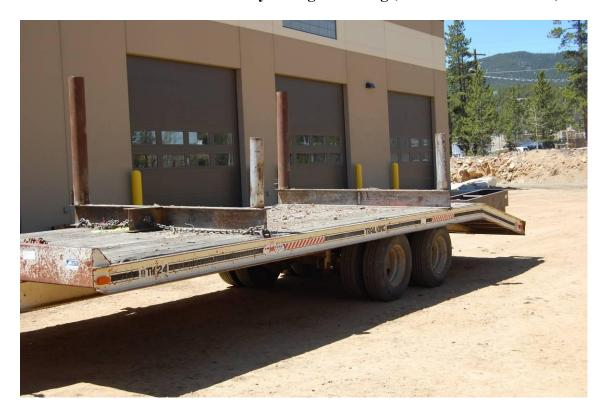
Min. 8' between risers, risers should be 8" high to allow unloading (below)
